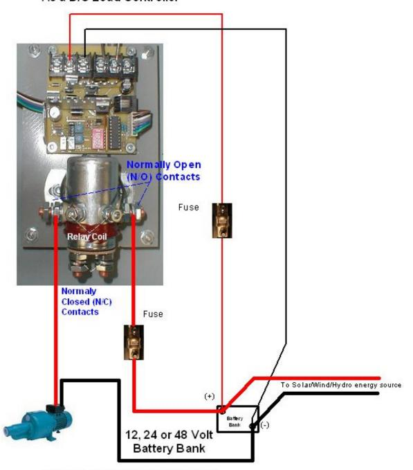
In this mode, the D/C input to the pump will only be connected if and when the battery reaches the user settable upper trip point.
