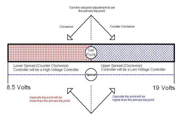
Voltages reflect a 12-volt system; double this for 24-volt systems, quadruple for 48-volt systems.
