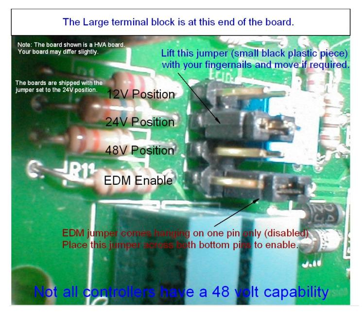
Note: Position 4 is the EDM jumper on versions 3.2 (EDM) and later. If you elect to use EDM, install this jumper in addition to the voltage selection jumper. You will always select a particular voltage, regardless if you elect to use EDM or not. EDM is discussed in detail later in this manual.
