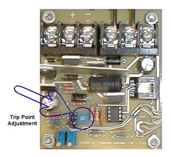
The controller has already been calibrated by the factory using the following settings, and does not require calibration, unless the trip point used is not satisfactory for your installation.
